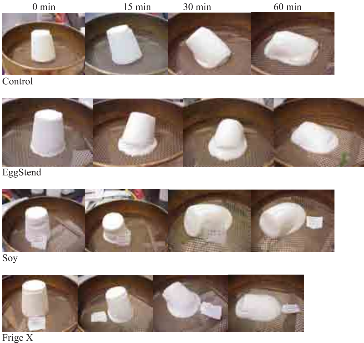
Figure 7.5 Representative image of comparing the melting properties of French Vanilla ice cream formulated with either egg yolks or egg alternatives over 60 min at room temperature.
