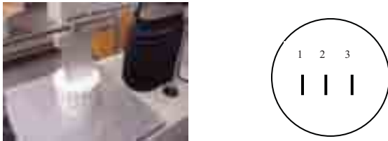
Figure 7.3 Depiction of the set-up and measurement locations used to measure the French Vanilla ice cream treatments hardness.
